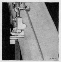
Fig. 51. Piping with the Edge-Stitcher
