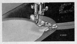
Fig. 44. Binding an Outside Curve
