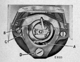
Fig. 27. Showing Position of Shuttle for Removal from Machine
