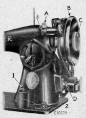
Fig. 5. Winding the Bobbin
