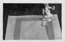
Fig. 52. Applying Bias Folds with the Edge-Stitcher
