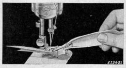
FIG. 41. INSERTING BINDING IN BINDER
