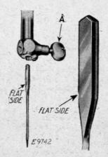
Fig. 11. Positioning of Needle in Needle Clamp
