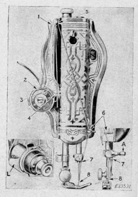
Fig. 12. Upper Threading
