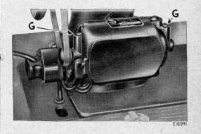
Fig. 26. Lubricating the Motor
