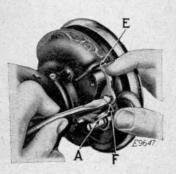
Fig. 6. Adjustment of Bobbin Winder
