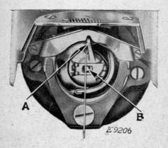
FIG. 10. BOBBIN CASE THREADED AND REPLACED
