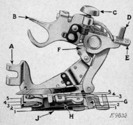
FIG. 59. THE RUFFLER AND ITS PARTS
