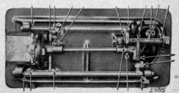
Fig. 25. Oiling Points in Base of Machine
