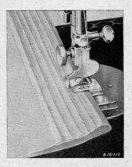
Fig. 55. Tucking with the Edge-Stitcher
