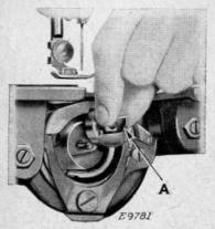
Fig. 4. Removing the Bobbin Case
