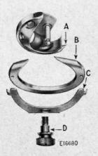
Fig. 28. Shuttle and Parts Removed from Machine
