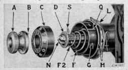
Fig. 20. Reassembling and Replacing the Tension
