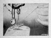
Fig. 13. Drawing Up Bobbin Thread
